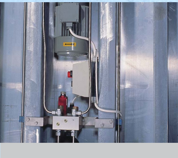
Hydraulic system, type Power Pack, mounted on horizontal plate freezer
