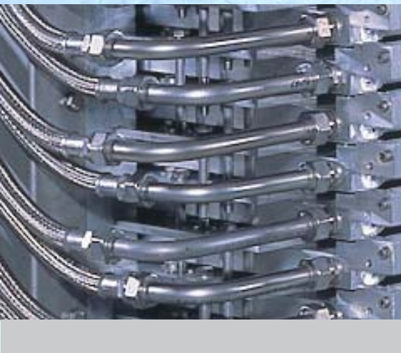
Flexible PTFE hoses, for R22, stainless steel-armoured individually pressure tested. Stainless steel bellow hoses for R717, individually pressure tested. Stainless steel fittings.
